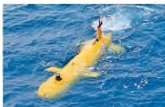
AUV (autonomous underwater vehicle; 自律型無人潜水機)
